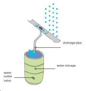
**F.60 Figure 60:** Diagram showing how a water butt works.
