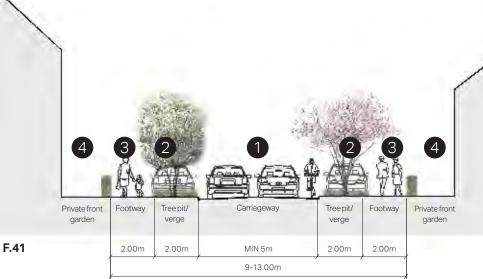
Figure 41: Cross-section to illustrate a residential street.
