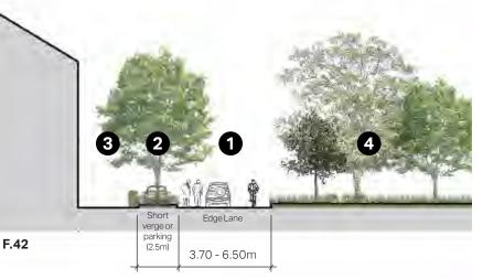
Figure 42: Cross-section to illustrate some guidelines for edge lanes.
