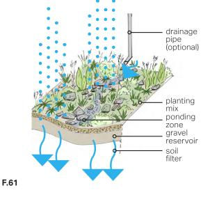
Figure 61: Diagram showing how a rain garden works.
